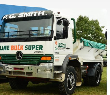
Our roll over tarp system is a simple, heavy duty and very effective tarp system which can be made from Mesh or Waterproof PVC. It operates by rolling a roll tube that uncovers a tarp across the width of the bin. Kiwi Tarp roll over systems are 100% kiwi made which feature nothing but the best quality components and materials in all our systems.
